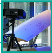
Setup of the VAS System projecting onto an Eurofighter Airbrake
