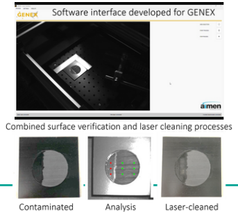
Combined LIBS module and laser cleaning. Control and analysis GUI detects contaminated areas. Processed samples were contaminated and correctly analyzed and cleaned.
