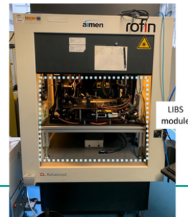
Combined LIBS module and laser cleaning. Control and analysis GUI detects contaminated areas. Processed samples were contaminated and correctly analyzed and cleaned.
