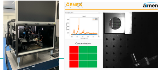
(Left) Stand-alone and out-of-the-lab LIBS system implementation; (Right) Software interface for control and LIBS analysis
